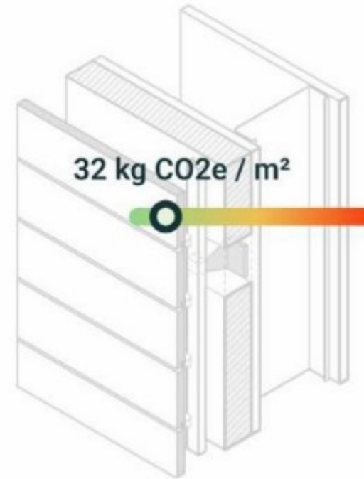
Wood facade cladding
